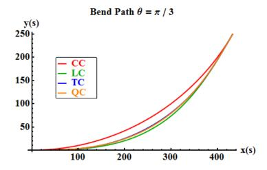
FIGURE 9. Bend paths for the constructed CC, LC, TC and QC curves. All bends start and finish at the same position. The variable curvature bends have slightly longer path-lengths  $L_{cc} = 523.6$ ,  $L_{lc} = 538.1$ ,  $L_{tc} = 534.6$ ,  $L_{ac} = 535.0$ .
