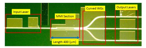
FIGURE 1. Photonic Integrated Circuit (PIC) containing curved optical waveguides [8].
