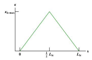
FIGURE 4. Curvature profile associated with a linear curvature bend
