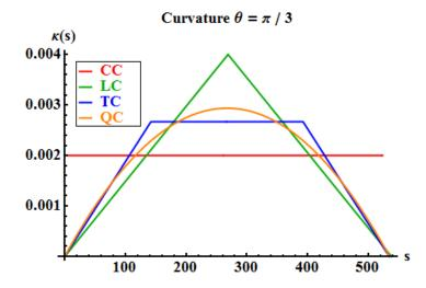
FIGURE 7. Curvature profiles for the constructed CC, LC, TC and QC curves.  $\kappa_{cc} = 0.002, \kappa_{lc}^{max} = 0.004, \kappa_{tc}^{max} = 0.0027, \kappa_{qc}^{max} = 0.0029.$
